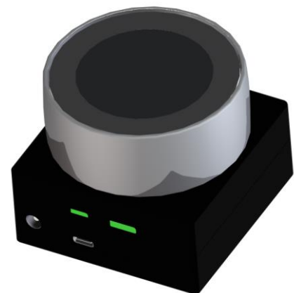
Smart knob mounted with 2x screw M3 x 8 mm to the case
